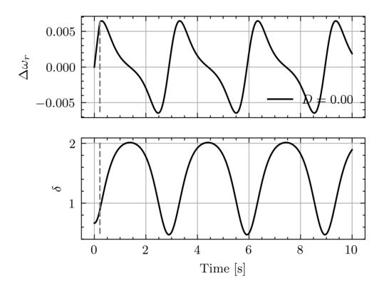
The fault is cleared after 214 ms (lower bound on the clearing time). As expected from previous calculations, the system is safe.
