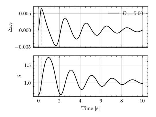
The fault is cleared after 239 ms (upper bound on the clearing time). The system is stable thanks to the damping effect (energy dissipation).
