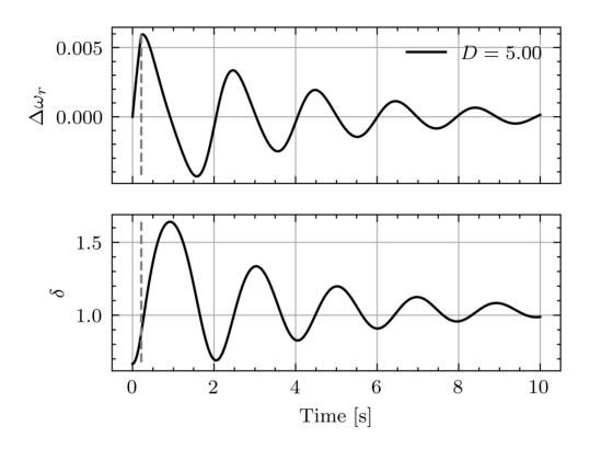
The fault is cleared after 214 ms (lower bound on the clearing time). As expected from previous calculations, the system is safe. The damping adds energy dissipation, which allows the system to stabilize around  $\delta_2=1.028$
