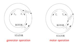
In synchronous machines, the rotor rotates at the same angular speed as the magnetic field produced by the stator. If we denote  $\omega_m$  the rotor angular speed and  $\omega_s=2\pi f_s$  the synchronous speed, then  $\omega_m=\omega_s$ .
