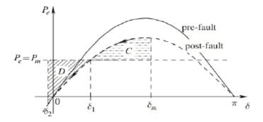
Without any damping (kinetic energy losses), the system oscillates indefinitely between angle  $\delta_2$  and  $\delta_m$ .
