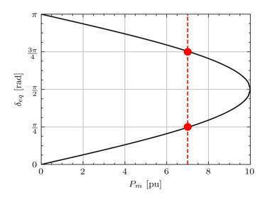
When we increase  $P_m$ , the electrical angle at equlibrium also increases. The maximum value is reached for  $\delta_{eq}=\frac{\pi}{2}.$
