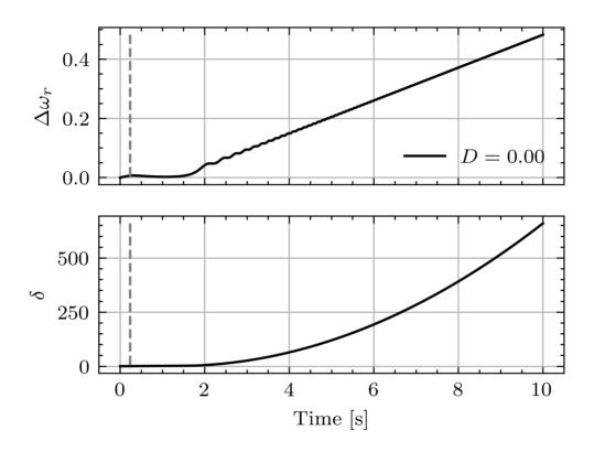
The fault is cleared after 239 ms (upper bound on the clearing time). The machine loses synchronism.
