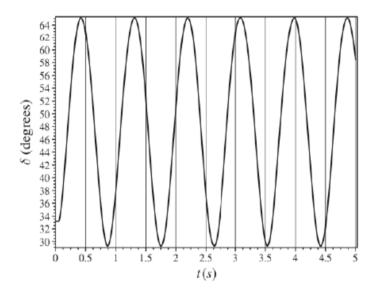
However, in a real system, the damping would cause the machine to settle down at an angle  $\delta_1$  (new equilibrium point).
