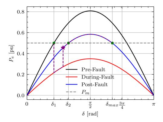
The purple star corresponds to  $\delta_{cct}=0.8938$ , and the dashed purple line shows the evolution of the angle  $\delta$ . Even without damping, the system stabilizes at  $\delta=\delta_{max}$  since the kinetic energy reaches 0 at that point ( $\Delta\omega^2=0$ )
