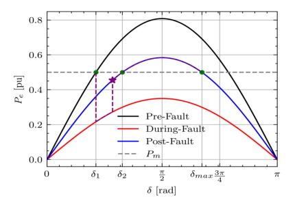
it is clear that the acceleration is maximum for  $\delta=\delta_1$ , and minimum for  $\delta=\delta_{cct}$  for  $\delta\in[\delta_1,\delta_{cct}]$  (larger power mismatch when  $\delta=\delta_1$  and smaller for  $\delta=\delta_{cct}$ ).
